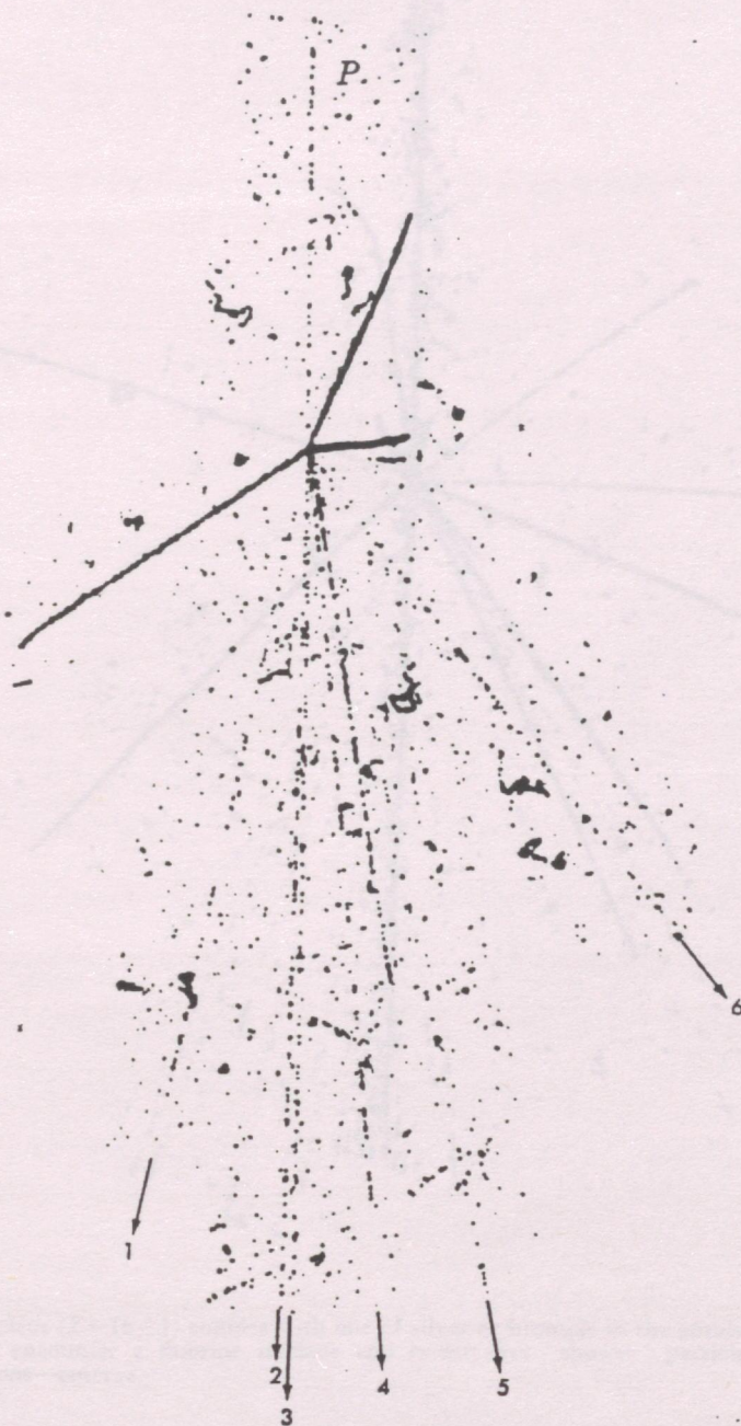
A Proton or a Pi-meson collides with a Silver or Bromine nucleus of the emulsion and produces 6 high energy secondaries and 3 heavy fragments.
