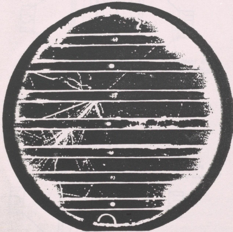
Photograph of a nuclear interaction produced by a penetrating particle underground (190 m.w.e.). The heavily ionizing particle coming out of the third plate and going to the left edge of the photograph may be a heavy unstable particle which has stopped and decayed in the fourth plate. The secondary particle probably stops in the last plate after penetrating two plates. Local gas turbulence has distorted the other heavily ionizing track in the third compartment.
