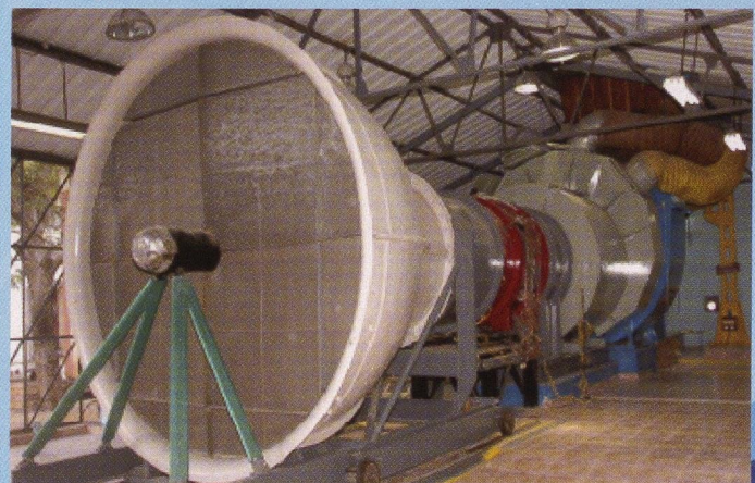
Test Rig for Turbine and Compressor Aerodynamic Investigations
