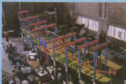
Static Structural Testing of SARAS wing.
