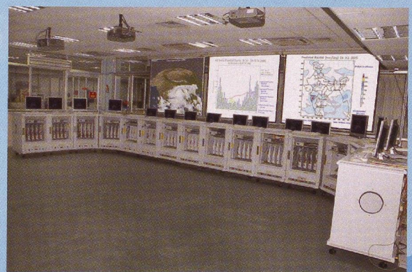
The 128 processor Flosolver Mk 6 and the results of computations made using the Varsha GCM.
