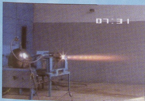
Zirconia based ceremet convergent-divergent nozzle being tested.
