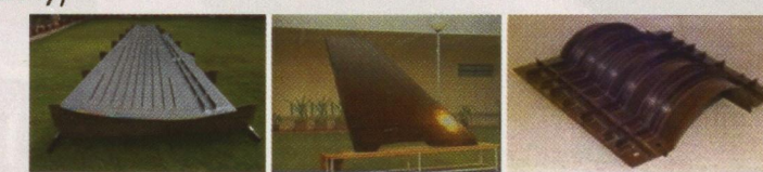
SARAS wing, torsional box and trouser duct-top for LCA
