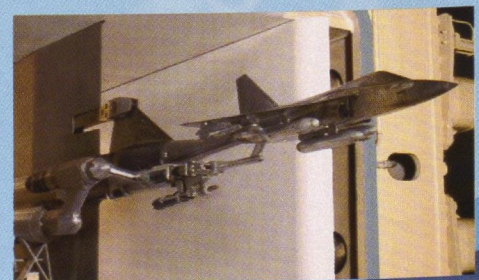
Captive Trajectory system for studies on stores separation from aircraft models.
