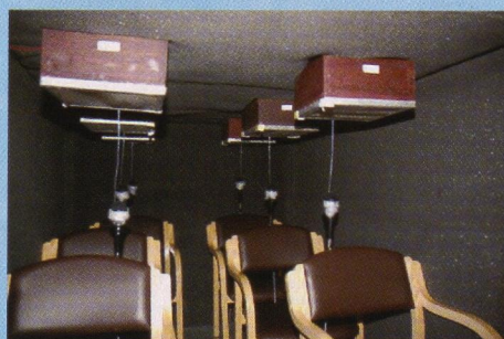
ANC setup inside the enclosure.
