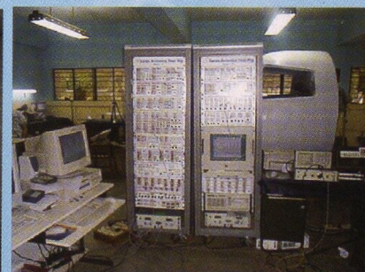
Avionics Ground Test Rig for integration testing of SARAS Avionics suite.
