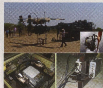
SHM system assembled on Nishant Wankel
