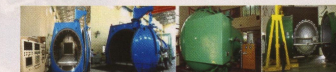
Mark IV Mark III Mark II Mark I Industrial grade, high temperature (350°C) and high pressure (15 bar) autoclaves for demanding applications
