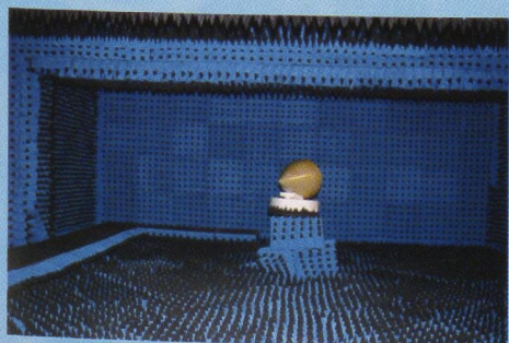
NAL-Microwave Anechoic Chamber (NAL-MAC).
