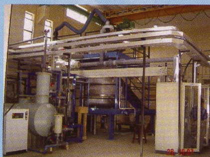
Isothermal Chemical Vapour Infiltration reactor facility established at NAL.
