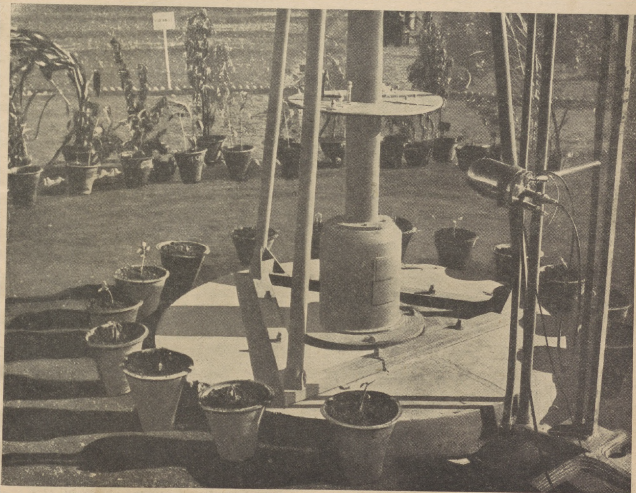
A close-up of the Gamma source with the seed tray and the monitor used for measuring radiation
