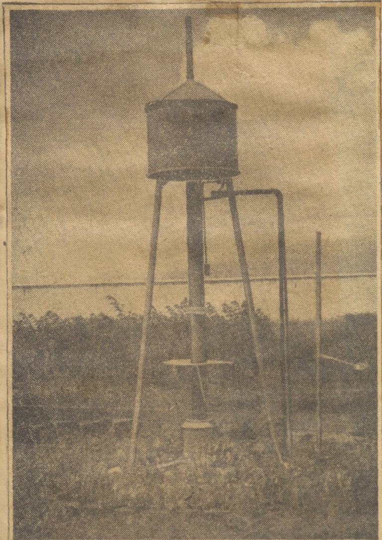
A view of the Gamma garden at Pusa, with the tower housing the source of radiation and its hoisting mechanism in the foreground.
