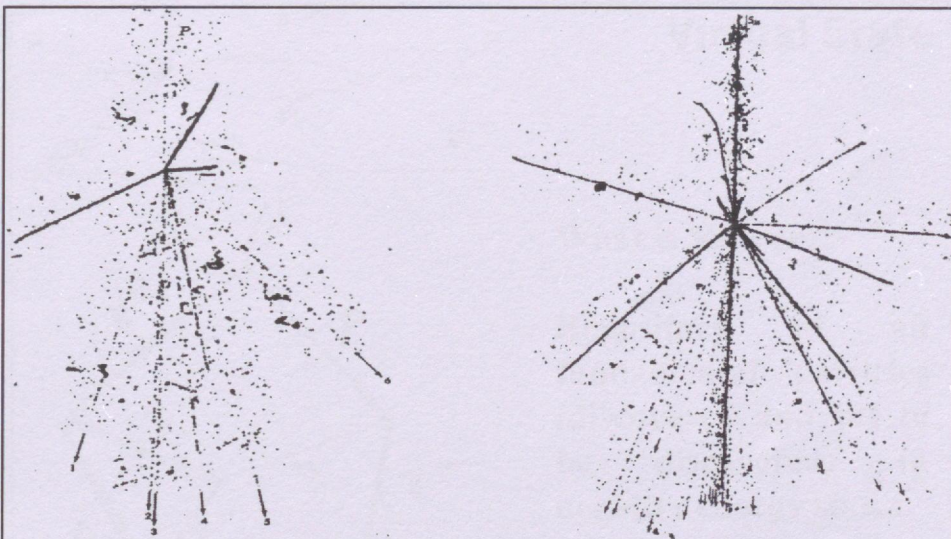
A Proton or a Pi-meson collides with a Silver or Bromine nucleus of the emulsion and produces 6 high energy secondaries and 3 heavy fragments.
