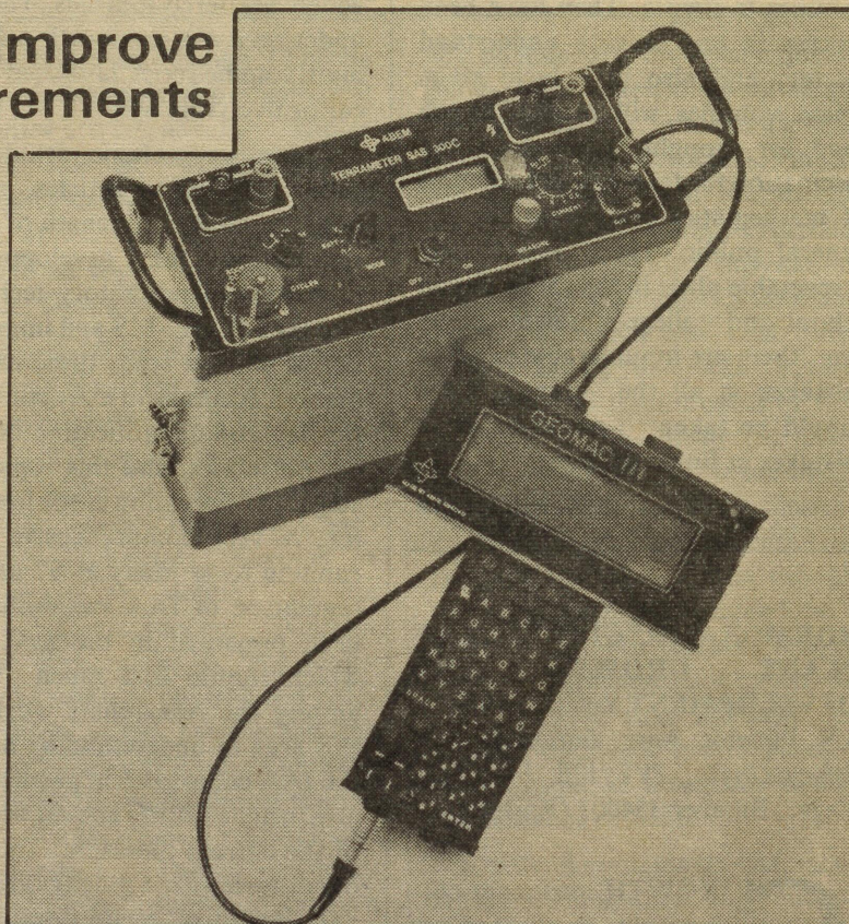
Hand-held computer for geological resistance measuring
