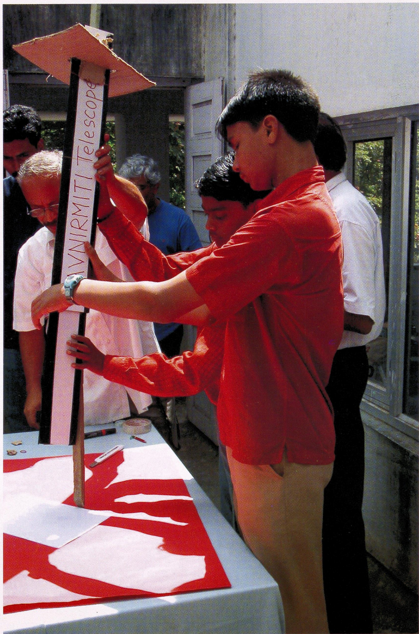
Plate 5. The low cost telescope is made with mountboard and two lenses.
