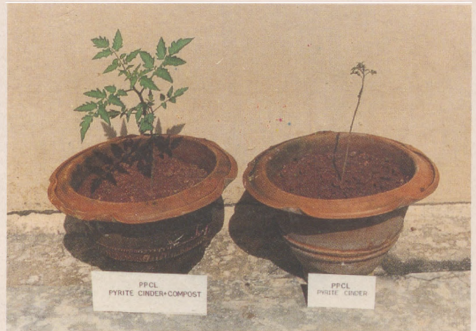
Fig. 70 Experiment showing the comparison of growth of plants in original pyrite Cinder and amended pyrite Cinder at CME, Dhanbad
