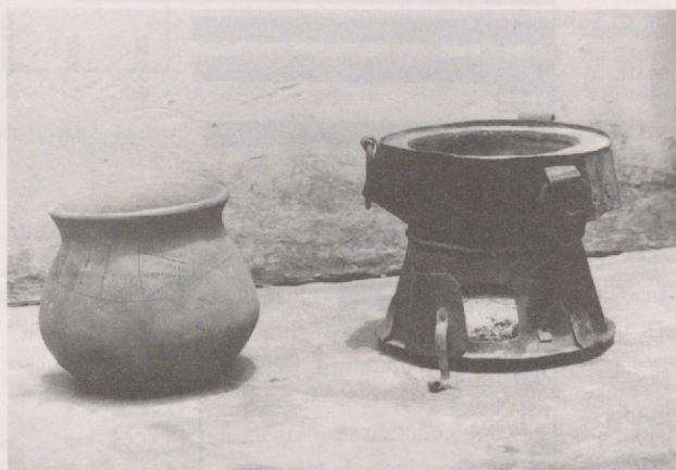
Figure 1b: Photo/D.M. Kammen Kenya Ceramic Jiko (right) Cooking pot (left)
